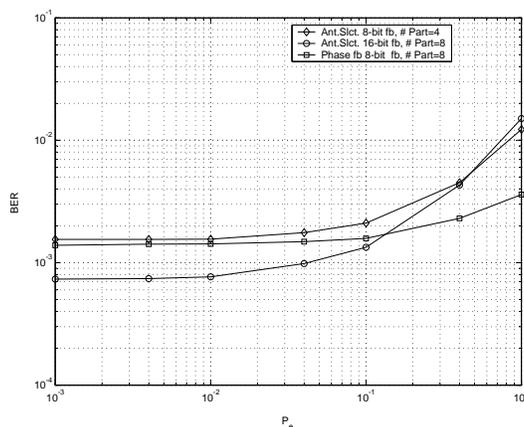
Fig. 5. BER performance comparison of the proposed algorithms with respect to the feedback error rate. Both algorithms are almost unaffected from feedback error upto  $P_e=10^{-2}$ , making them robust against feedback errors. The antenna selection algorithm appears to be more vulnerable for high  $P_e$  values compared to the phase feedback algorithm.
