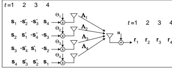
Fig. 1. The proposed system model with four transmit and one receive antennas. The QO-STBC to be transmitted is depicted on the left hand side besides the weighting of the antennas used in the proposed algorithms. The channel coefficients  $\Lambda_i$  are the effective flat-fading representations of  $h_i[n]$  after frequency domain transformation.
