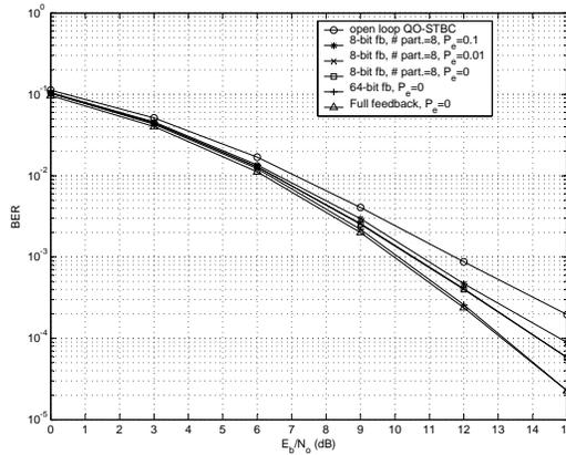
Fig. 3. BER performance comparison of the phase feedback algorithm when exposed to quantization and feedback errors. Only one bit feedback performs almost equally well as the full feedback scheme. Also the phase feedback algorithm is very robust against feedback errors and the effect of feedback error rate of  $10^{-2}$  is negligible.
