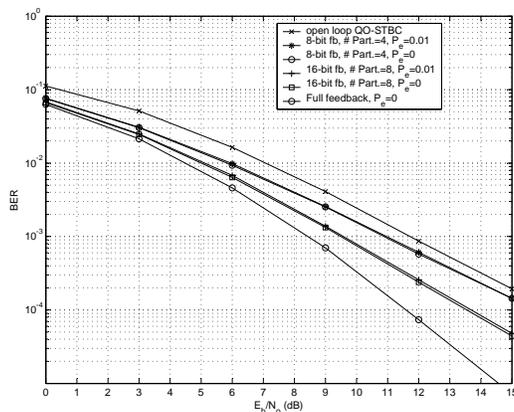
Fig. 4. BER performance comparison of the antenna selection algorithm when exposed to feedback errors. This algorithms appears to be more vulnerable to partitioning however it performs better than the phase feedback algorithm for moderate number of feedbacks, 16-bit in this simulation. The antenna selection algorithm is also very robust against feedback errors and the effect of feedback error rate of  $10^{-2}$  is negligible.
