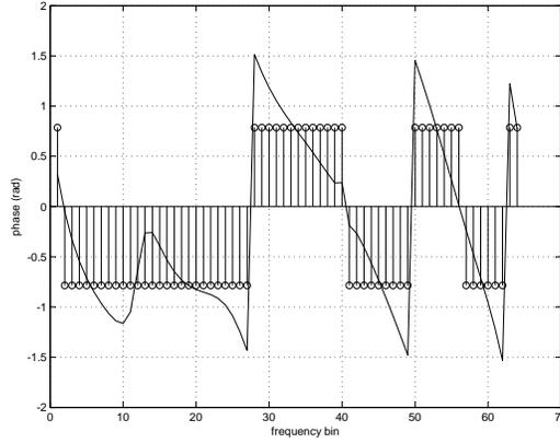
Fig. 2. An illustration of the feedback information. For the phase feedback algorithm, the actual phase values is shown with solid lines, whereas the ‘stem’ is the corresponding one-bit quantized phase value. Observe the strong correlation between adjacent bins. The same behaviour is also observed for the antenna selection algorithm.
