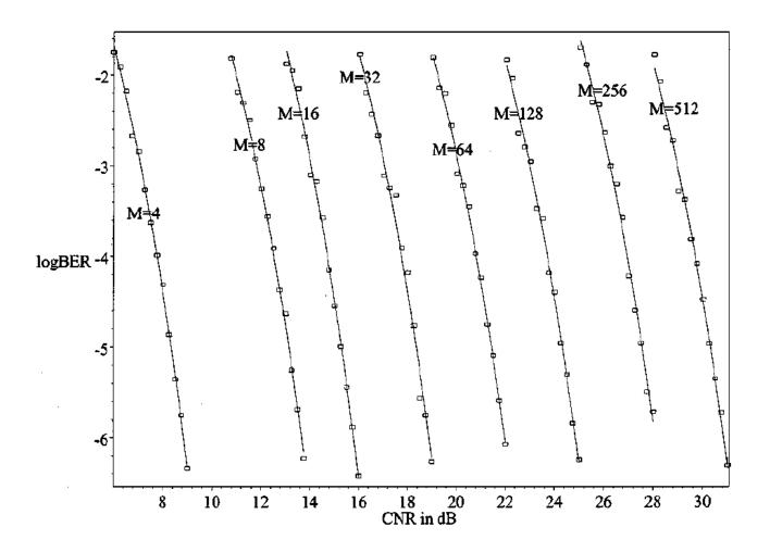
Based on: "Adaptive Multidimensional Coded Modulation Over Flat Fading Channels", K. J. Hole, H. Holm and G. E. Øien
