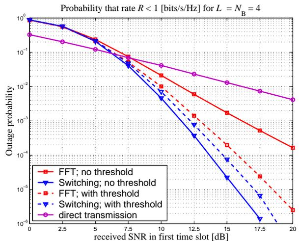
Fig. 4. Outage probability that the rate is less than 1 bit/s/Hz for  $L = 4$  relays and block-length  $N_B = 4$ ; with threshold  $a_{\max}$  (dashed lines); no threshold (solid lines); direct = no relays, source sends in every time slot
