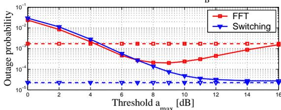
Fig. 3. Outage probability that the rate is less than 1 bit/s/Hz vs. threshold  $a_{\max}$  for  $L = 4$  relays and block-length  $N_B = 4$ ; with threshold  $a_{\max}$  (solid lines); no threshold (dashed lines);
