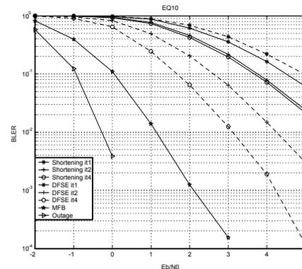
Fig. 1. Block-static MIMO system  $2 \times 2$  EQ-10
